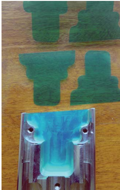
Making masks by unreliable manual methods (left) is increasingly replaced today with computer-design of custom masks and diecuts.
